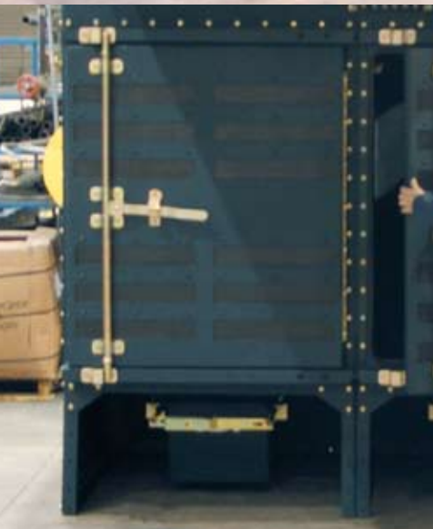
21,600 CFM Gold Series Booth encapsulates blast dust in countertop manufacturing area.
