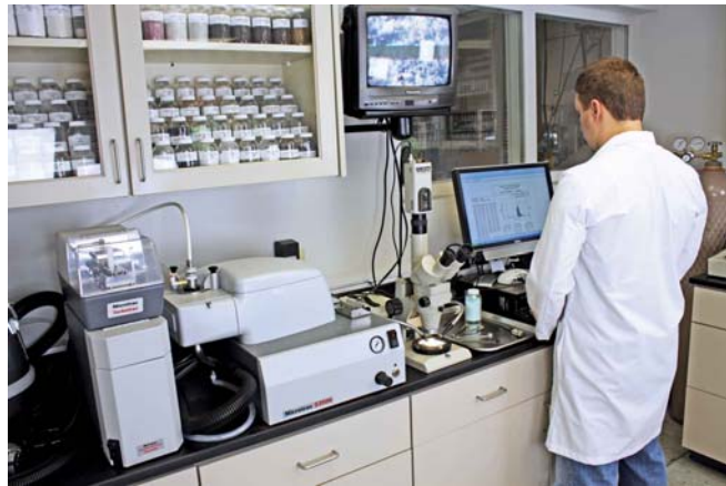
Particle-size analysis is used to reveal dust's particle-size distribution down to the submicron range.
