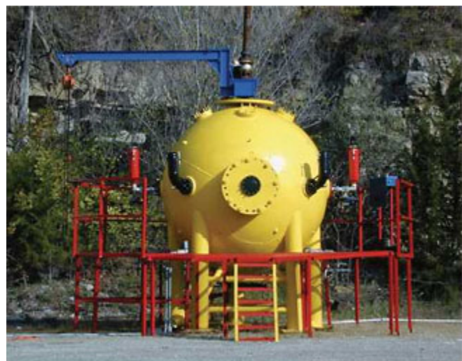
When advanced testing is needed on combustible dusts, full-scale explosion test vessels can be used. (Fike Corp.)
