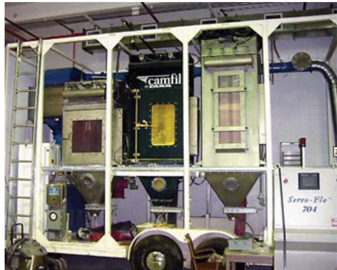
Test rig using multiple dust collectors to perform specialized full-scale dust testing.
