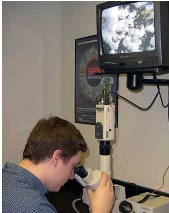
A video microscope provides visual analysis of dust shape and characteristics.
