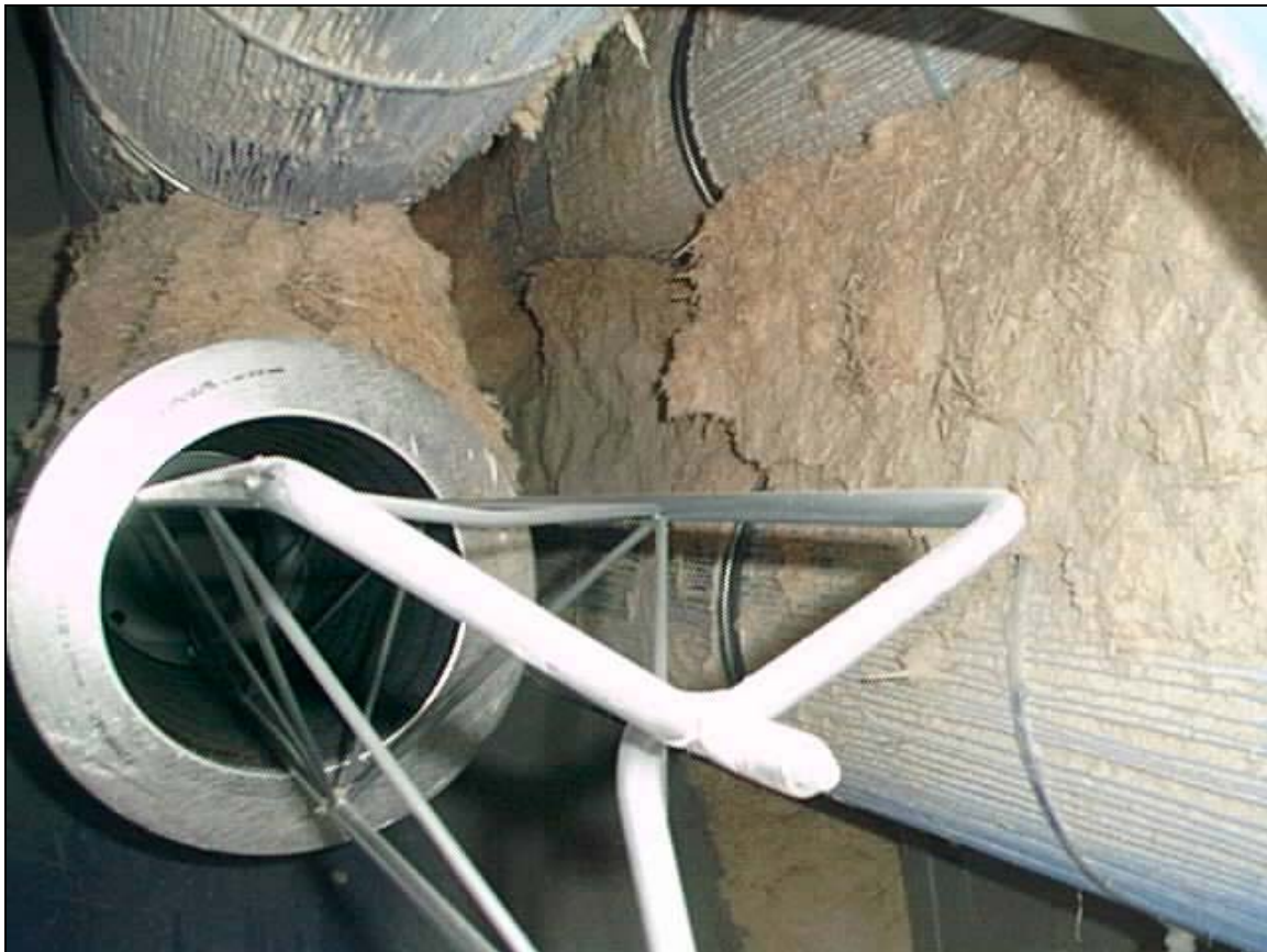
Fig. 1 Filters lying on their side results in top loading of the filter cartridges.
